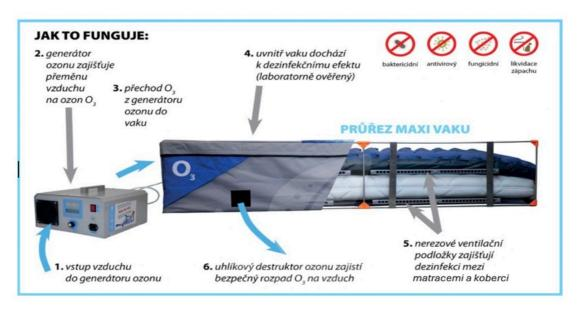
Ozone disinfection cleaning is completely environmentally friendly, as it uses no chemicals or harmful substances. Ozone naturally breaks down into oxygen, so there are no chemical residues or toxic substances left after cleaning that could negatively affect the environment or your health. Here are the deep dry vacuum ozone cleanings:
